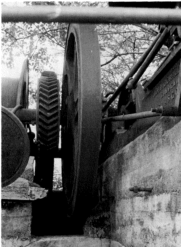
Fig. 9: Flywheel and helical gears, Iguana Consols winding engine. Dial indicator on left.
