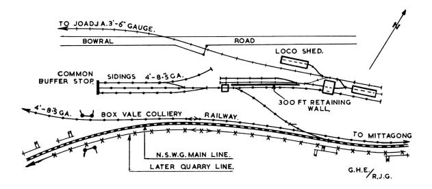
and lack of engine run-round facilities, would have proved most difficult to shunt and one can only surmise that recourse to much gravitation of the vehicles had to be made, also the constant use of a tow-rope and push-bar. It is also possible that the services of a shunting horse may have been necessary.
