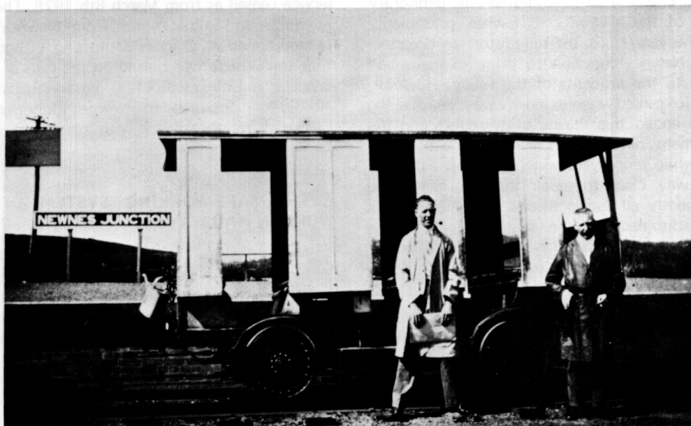
The rail motor as rebuilt to provide protection against the winter elements.
