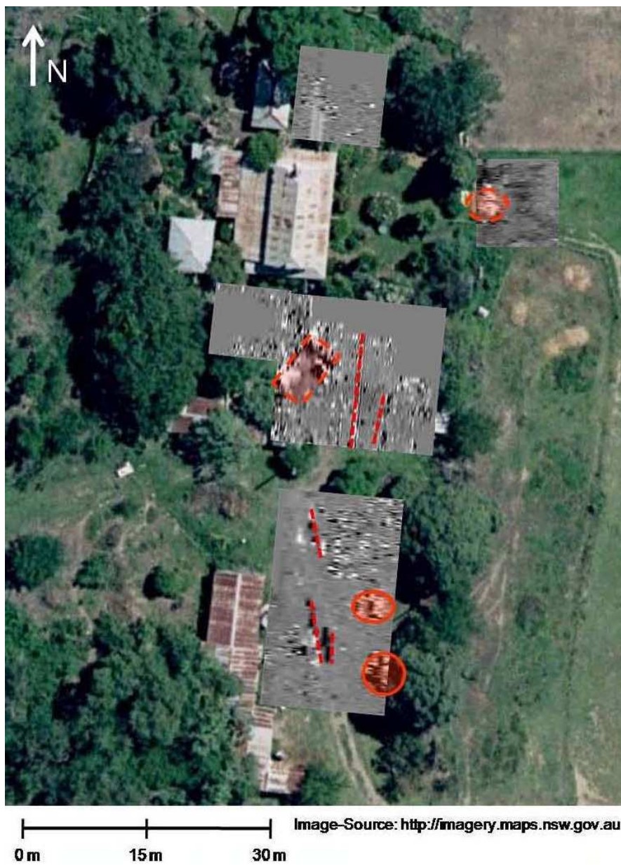
Figure 25 Ground Penetrating Radar (GPR) image showing location of former structure (dashed rectangle), silage pits (circles) and services (dashed lines). (Source: Archaeological Computing Laboratory, University of Sydney)
